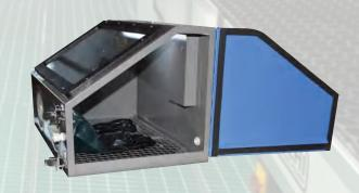
Another useful accessory is the completely hermetic box, the MI Iron Box, a structure closer to a sandblaster, with a frontal glass to check the production, gloves to grab the workpieces and an external light.
