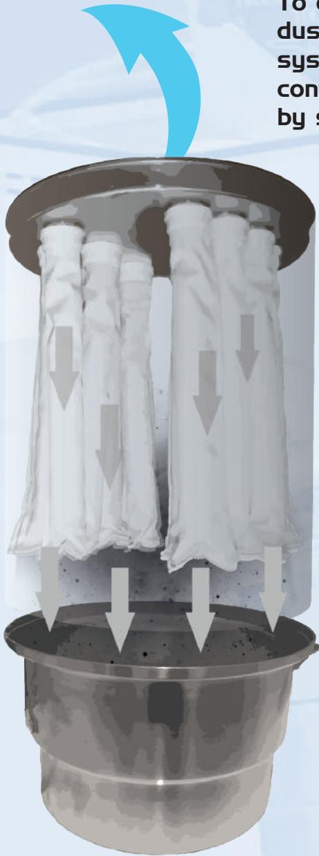
To effectively clean the filters mounted on the dust extractor, a mechanical shaking cleaning system has been developed. The electronic board controls automatically a pneumatic piston which, by shaking the filter intensely, causes, to the dust deposited filter, to fall into the powder container, thus allowing the filter to run optimally.
