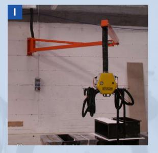
THE HEXAGON-SHAPED SERVICE CONTROL UNIT IS THE IDEAL PRODUCT AS A TERMINAL OF THE ARTICULATED ARMS (I) BUT ALSO AS A PENDANT SATELLITE (2) AND FOR THE INSTALLATION IN WALL (3).
