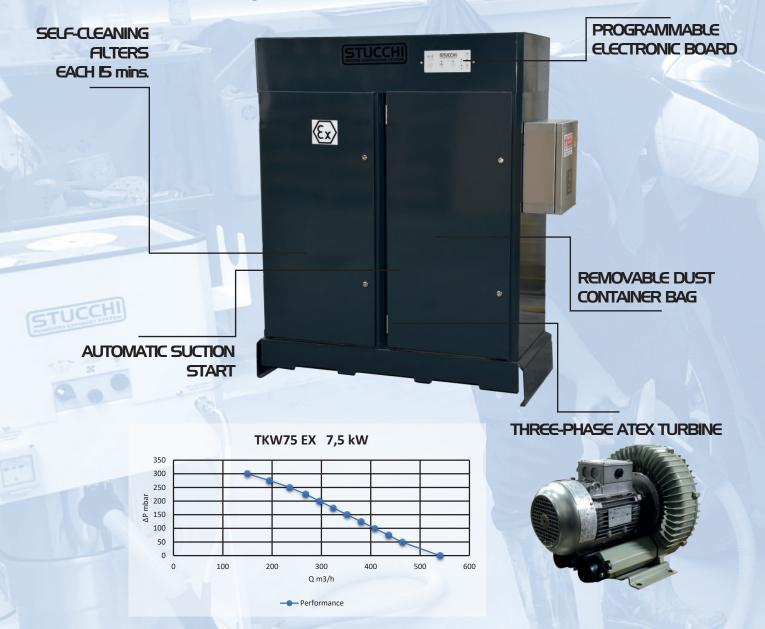
All vacuum cleaners prevent the formation of static electricity, overheating of the motors and other devices.
