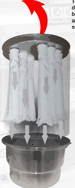
To effectively clean the filters mounted on the dust extractor, a mechanical shaking system has been developed. The electronic board controls automatically a pneumatic piston which, by shaking the filter intensely, causes, to the dust
