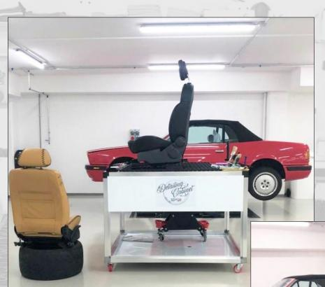
Thanks to the detailing bench it is possible to carry out aesthetic works on previously disassembled components, without having to dirty / damage the other parts of the vehicle.
